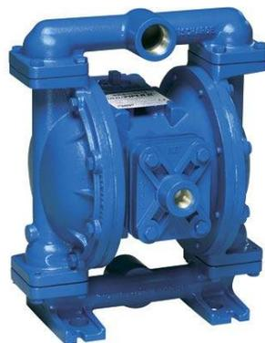
*Our specially designed Sandpiper Pump is C.S.A. certified to operate off of a gas or air supply, which is a readily available product at most oil and gas locations. Our pump is rated at 44 GPM at 80 psi. Most pumps use rubber balls and seats along with Buna O-rings inside the air motor, while ours uses Nylon balls and seats along with Viton O-rings. This keeps our pump operating while others on the market are at the rebuild shop.*
